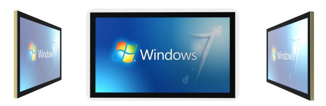
WTM270TL is an commercial grade PCT multi-touch touch monitor. It applies flat panel design, offers wide viewing angles and clear, crisp images. Its unique penetration ability provides flat surface similar to iPhone and superior multi touch experience. All its hidden behind glass touch sensor advantages are achieved no wear life components, and can truly not afraid of dust, water and light performance from the principle.
